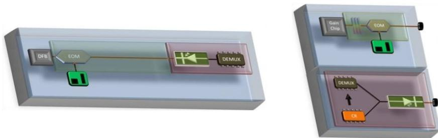
**Figure 1:** Artistic layout of POLYSYS system for 100 Gb/s chip-to-chip interconnect (left), and 100 Gb/s optical transceiver for 100 GbE telecom applications (right).
