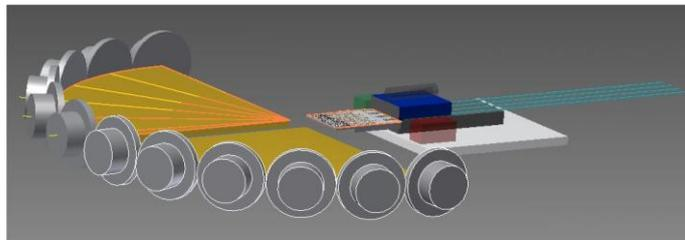
**Figure 3:** 3-D sketch of chip arrangement, optical coupling and network to output connectors of the planned 4x100 Gb/s photoreceiver module with DEMUX functionality (prepared by HHI).
