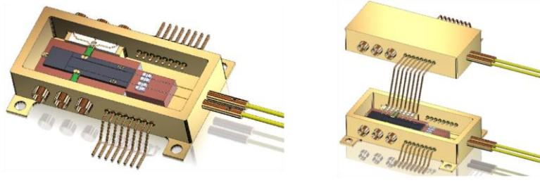
**Figure 2:** Layout of the 2x100 Gb/s transmitter (left), and of the arrangement for the twin 2x100 Gb/s module (right).
